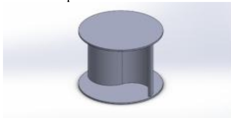
Gambar 2 Desain Turbin S-Shape
