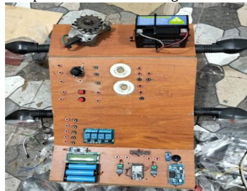
Figure 1 Display of the Motorcycle Electrical System Learning Media equipped with an AI and IoT-based monitoring system.
