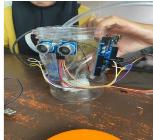
Image 2 Realization of automatic dispenser
